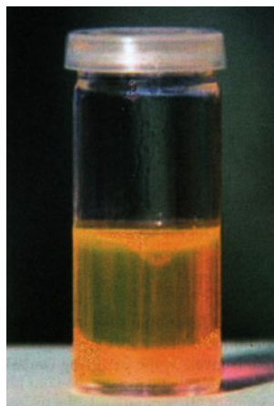
Fig. 1 A silica sol-gel system doped with a coloured organic molecule following Pagliaro
